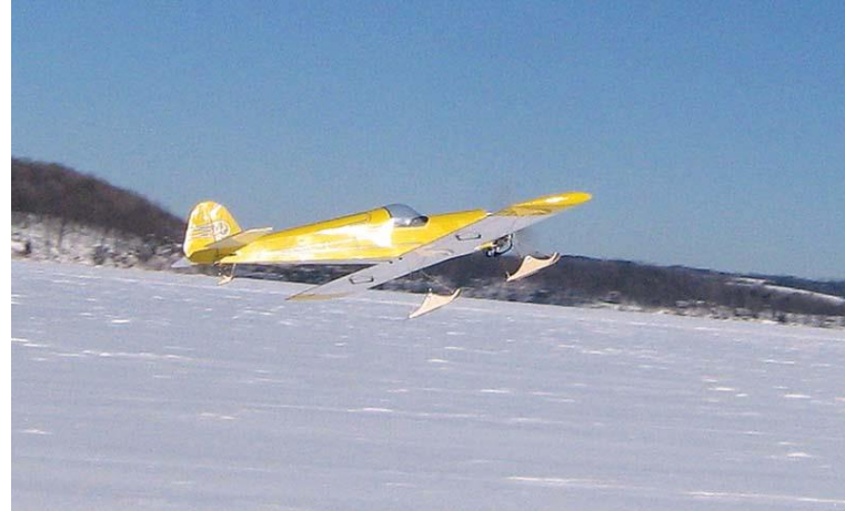
The Sky Wizard comes in for a snowy landing. Note that the tips of the skis are set at a positive angle.
